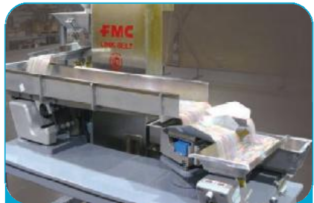
Integrated high stroke system using BF-3, RS drive, BF-2 and a Link-Belt bucket elevator.
